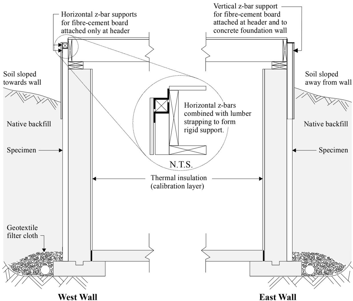
**Figure 1 Wall Sections Used in EIBS Field Testing**
