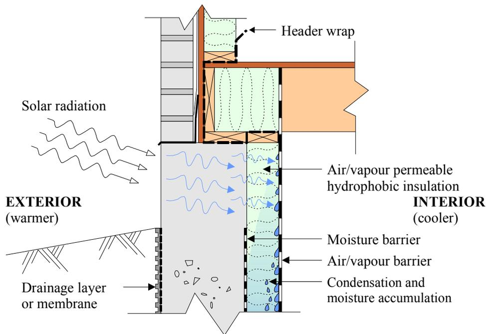
The dominant temperature gradient during summer months drives moisture entrained in the foundation wall inward, where it condenses on the outboard face of the air/vapour barrier. Much of the insulation and strapping normally reach saturation, and in some cases, bulk water runs out the bottom of the interior finished wall assembly (often mistaken for leakage).
